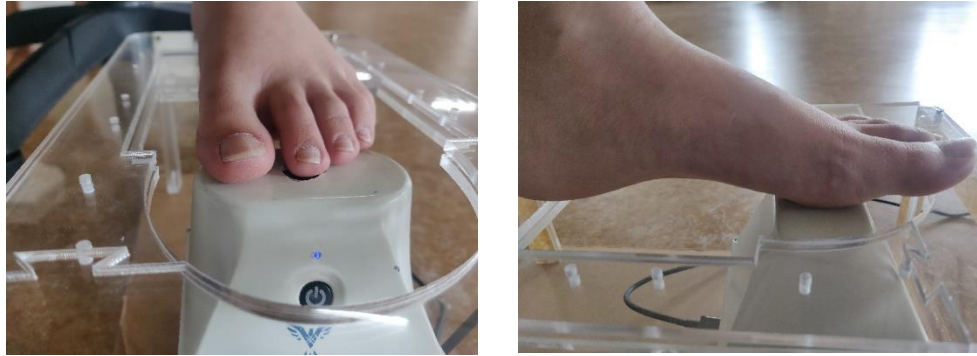
Figure 3: Device measuring plantar tissue stiffness at 1st metatarsal head and 2nd toe
